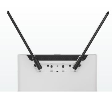
Chateau has two powerful (2x2 MIMO compatible!) integrated antennas, but you can connect two external LTE antennas (not included) for an even stronger signal.
