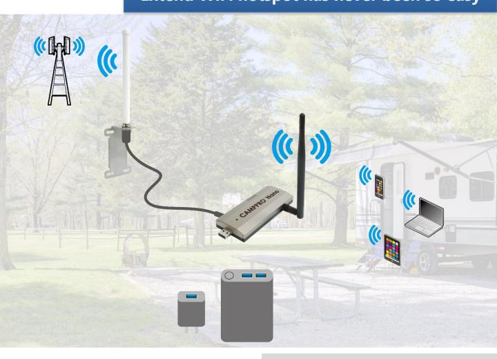
**WiFi CampPro Nano** is a dual-radio designed for retrieving and extending internet access in your house, mobile home, RV, or yacht from remote WiFi hotspots or home WiFi. Power the CampPro Nano by a power bank or USB DC adapter with the USB Type-A male connector. WiFi CampPro Nano has an extra USB port to support the 4G/5G USB modem with the 4G/5G carrier's data plan in the next firmware release.
