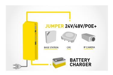
Thanks to smart Gigabit PoE supply every standard load such as PoE+, 802.3af & 802.2at devices, IP-Cameras, IP-Phones, PBXs, Access Point, Switches, CPEs, Routers, providing Output Voltage in case of black out. Output supply is selectable in continous way between 24V up to 52V.
