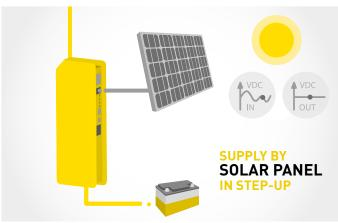
Easy to use Solar Panel. Work as step-up way and reserve energy on lower radiation. Integrated intelligent Power Management allow to optimize your systems using the battery charger. A great solution for video survelliance or wireless installation on street lamps.
